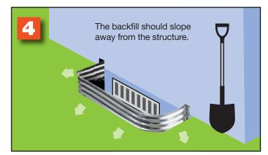
Add gravel to the well bringing the level up to 2" below the bottom of the vent opening. Backfill the area between the vent well and the hole.
