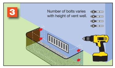
Drill holes to receive the anchor bolts, then secure the vent well to the foundation using anchor bolts and optional flat washers.
