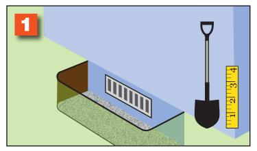
Pre-fill hole with at least 4" of gravel or drain rock to promote drainage. If flooding is a concern, connection to a perimeter drainage system might be required.
