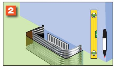
Position the vent well against the foundation and mark the location of the holes. Be sure the vent well is centered on the vent and level with the house.
