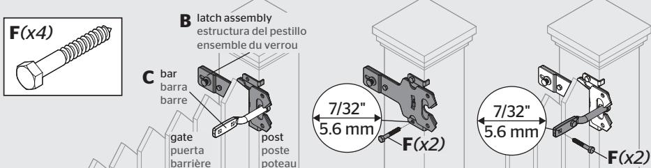
**C** Install pull on gate over bar. Make sure top screws install into frame rail.
