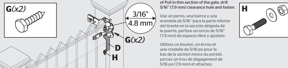
**D** Lock and unlock the latch assembly by moving the pin in the slot.
