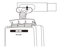
(5) Connect the window bracket to the window.
