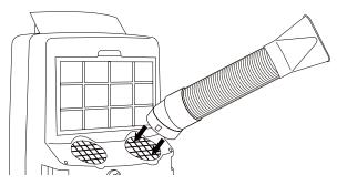
4 Connect the window bracket to the opposite end of the plastic hose. Ensure that all connections are tight and installed properly.
