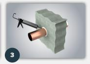
Apply caulking as required to close remaining gap to both sides of wall assembly; providing a smoke and gas resistant seal. Spread caulking smoothly and evenly all around.
