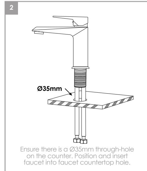
Ensure there is a Ø35mm through-hole on the counter. Position and insert faucet into faucet countertop hole.
