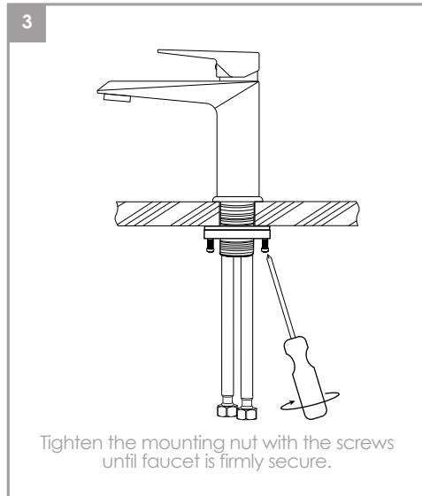
Tighten the mounting nut with the screws until faucet is firmly secure.
