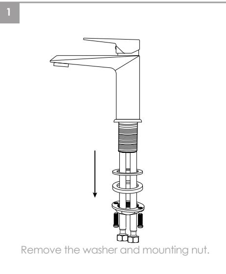
Remove the washer and mounting nut.
