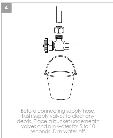
Before connecting supply hose, flush supply valves to clear any debris. Place a bucket underneath valves and run water for 5 to 10 seconds. Turn water off.
