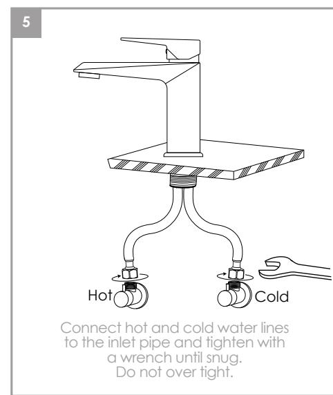
Connect hot and cold water lines to the inlet pipe and tighten with a wrench until snug. Do not over tight.
