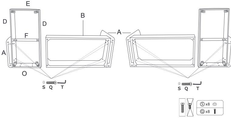
Step 2: Connect the Seat frame (B) to the Long board (D) with Washers (S) Butterfly nut (R) and Bolts (Q).
