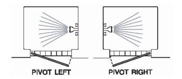
Note: This enclosure may be installed without using the sloped curb [A] provided. Its use is definitely recommended for positive water control on shower sills with little or no slope.
