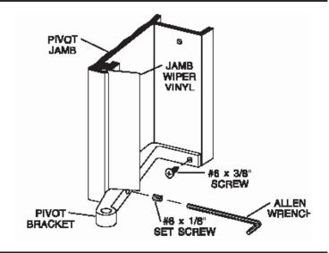
Place the pivot jamb [C] on the curb [A] with the exterior face lined up with the raised edge of the curb. Use a level to plumb the jamb then mark the mounting hole locations. Remove the jamb and drill the mounting holes.
