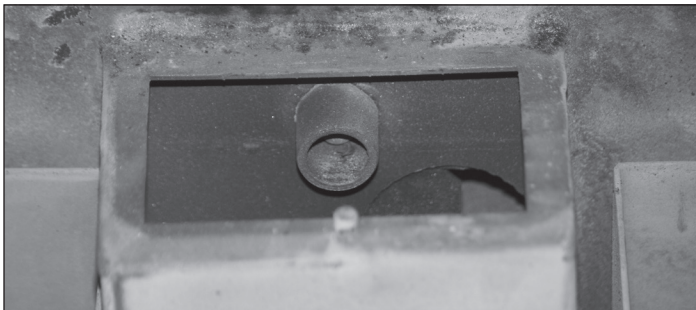
Figure 35: Remove ash from ignitor tube (underneath firepot)
