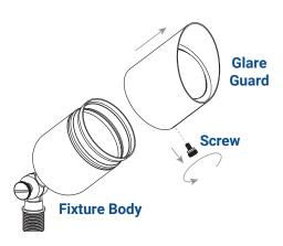
Loosen the screw and remove the glare guard from the fixture body.
