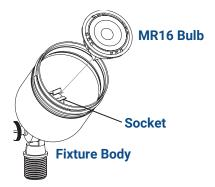
Insert MR16 bulb with correct wattage and type marked on fixture label.
