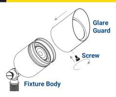
Place the glare guard back onto the fixture body and secure with previously removed screw.
