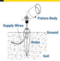
Pass supply wires through the center of the stake and thread the fixture body onto the stake.
