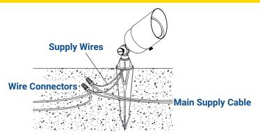
Strip two leads from fixture supply wires. Using two UL listed wire connectors (not provided), connect leads from fixture supply wires to main supply cable leads.
