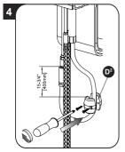
Attach the counterweight (D2) to the flexible hose approximately 15-3/4" [400mm] from the connection to the outlet pipe.
