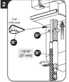
For countertop thicknesses less than 1/16" thick use the flange (B1), for all other installations use the metal washer (B2).
