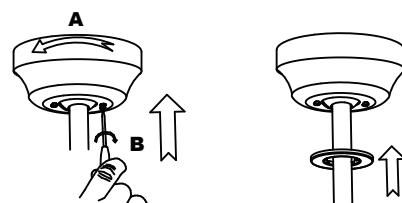
Slide the canopy up to ceiling and align the keyhole slots on the canopy with the 2 preassembled screws on the hanger bracket. Twist clockwise until it locks. Tighten two screws to fix the canopy securely. Clip the canopy cover in to secure it onto the canopy.
