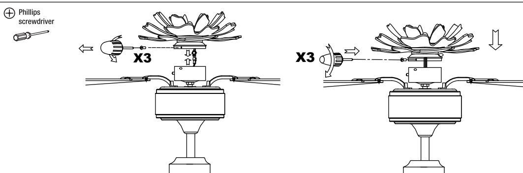
Remove 3 screws from the light kit, and then connect 2 connectors.
