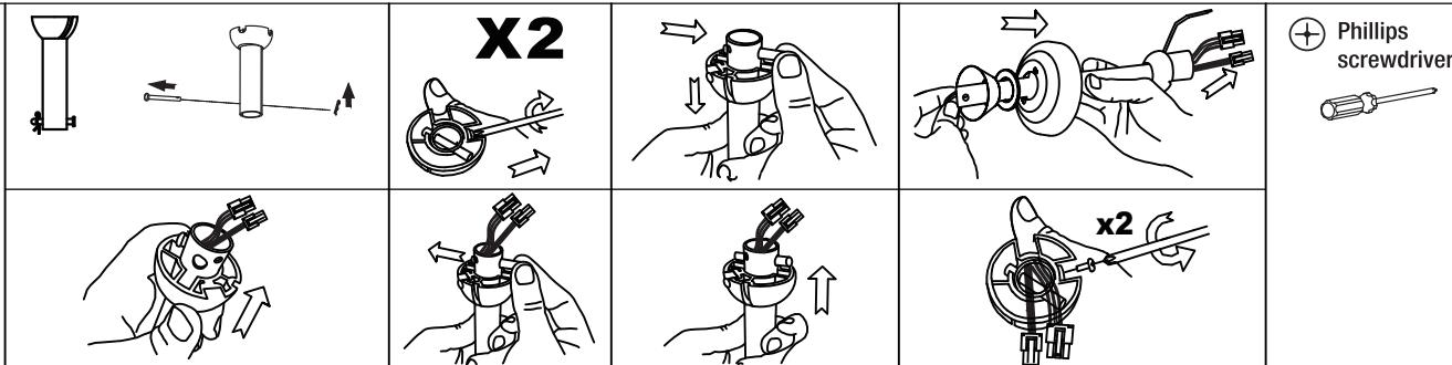
Remove the bolt, "R" lock pin and 2 set screws from the downrod and then take down the hanger ball.
