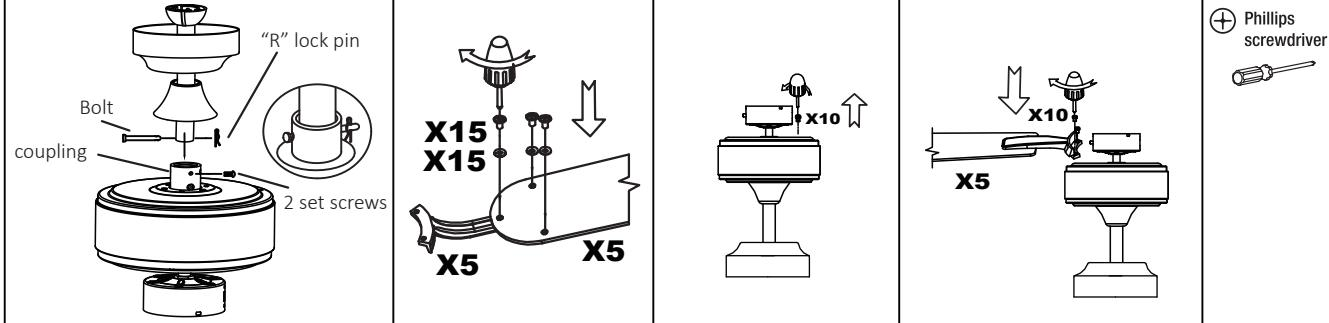
Insert the downrod into the coupling.
