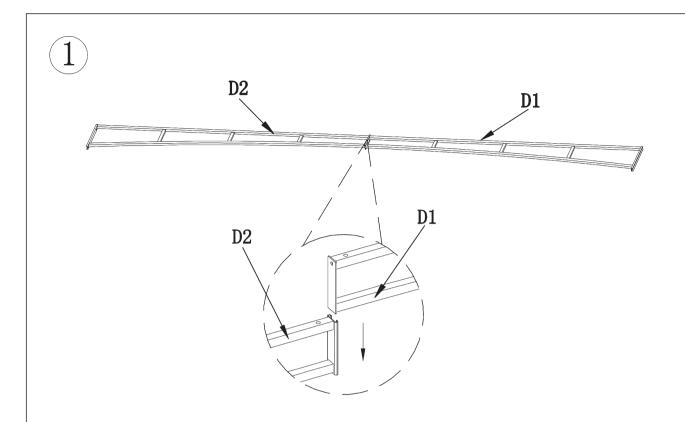
Connect two Long Side Beams(D1) to Long Side Beams(D2).
