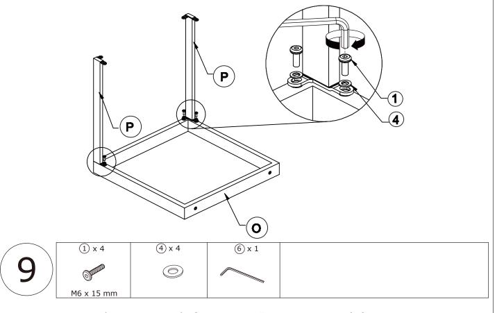
Fix part O with part P with four M6x15mm Screws (1) and (4) Flat Washers.Use (6) Allen key. **DO NOT YET TIGHTEN.**
