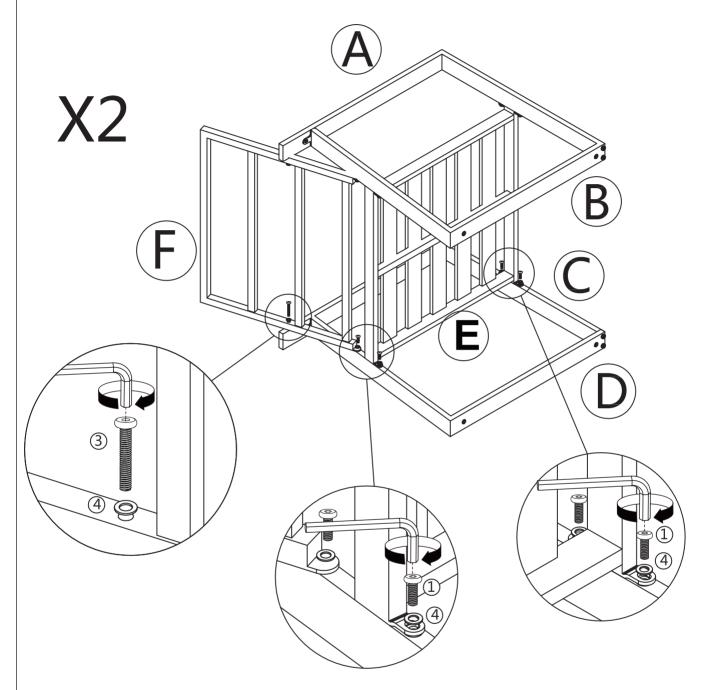
Fix part F with part C with one M6x35mm Screws (3) and (4) Flat Washers.Use (6) Allen key. **DO NOT YET TIGHTEN.**
