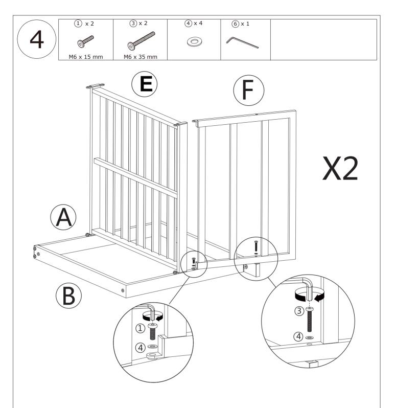
Fix part F with part A with one M6x35mm Screws (3) and (4) Flat Washers.Use (6) Allen key. **DO NOT YET TIGHTEN.**
