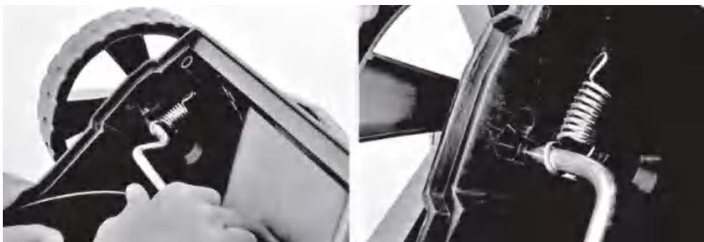
1600W lawn mower adjusts the three-level height of mowing by moving the wheel axle.
