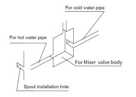
2.Recommended depth for installing shower valve body before tiling tiles: 40-50mm. Note: Tile opening should be bigger than shower valve diameter at least 5 mm.
