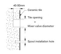
3.Connect water pipes to shower valve body as picture shows. And then install the shower valve body with screws.
