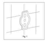
Place the mounting plate(s), Fig. 1, vertically at the corresponding location(s) on wall. Then, mark the screw holes locations on wall through the upper & lower holes at the mounting plate.
