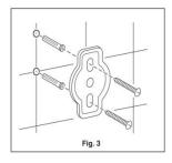
3) Push the plastic anchors provided into the holes until flush with wall. Then, screw mounting plates to wall with the screws provided, Fig. 3. Note: Molly or toggle bolts (not included) may be required for hollow wall.
