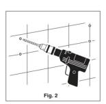
2) Take away the mounting plate. Drill holes at the marked screw locations, Fig.2. On ceramic tiles, try to locate screw hole(s) on grout line. If mounting on tile surface, use masking tape to do marking & to prevent sliding during drilling.
