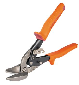
Cut and trim sheet metal in comfort with the Klein Tools left cutting Offset Snips. Snip blades are made of forged, heat-treated steel for strength and durability. Offset blades make it easier to cut in tight curves and keep the user's hand away from the metal. The contoured plastic handles with thumb guards are color-coded by cutting pattern.
