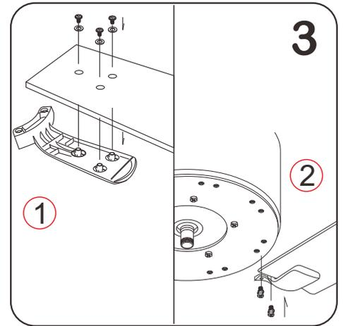
1. Match the fan blade hole to the fork and lock the screw as shown in the figure.
