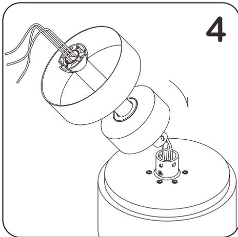
According to the figure, put the sponder into the upper cup, decorate the cover, and then thread the motor wire.
