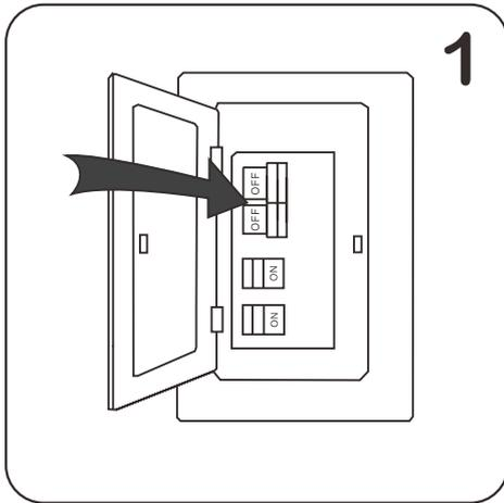
Turn OFF the electrical power at the main fuse of circuit breaker.
