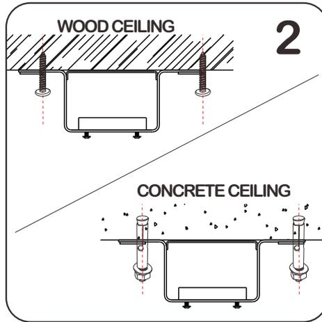
According to the different installation ceiling, select the corresponding installation screw for installation
