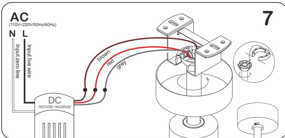
After hanging the fan sponder into the hanger, rotate and clip it into the groove, then connect the wires according to the color, and finally put on the hanging cup. After rotating the hanging cup, lock the hanging cup screw
