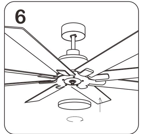
Screw the decorative cover clockwise into the motor shaft as shown in the figure, and make sure it is firm.
