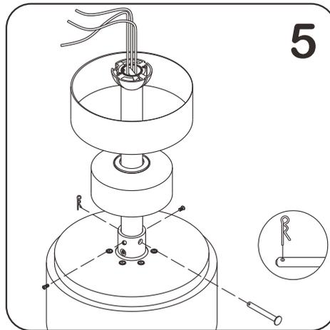
Clip the sponder into the fan motor, then rotate it to align with the hole, insert the cross bolt screw, lock the R pin, and finally lock the two screws on the hanger head.
