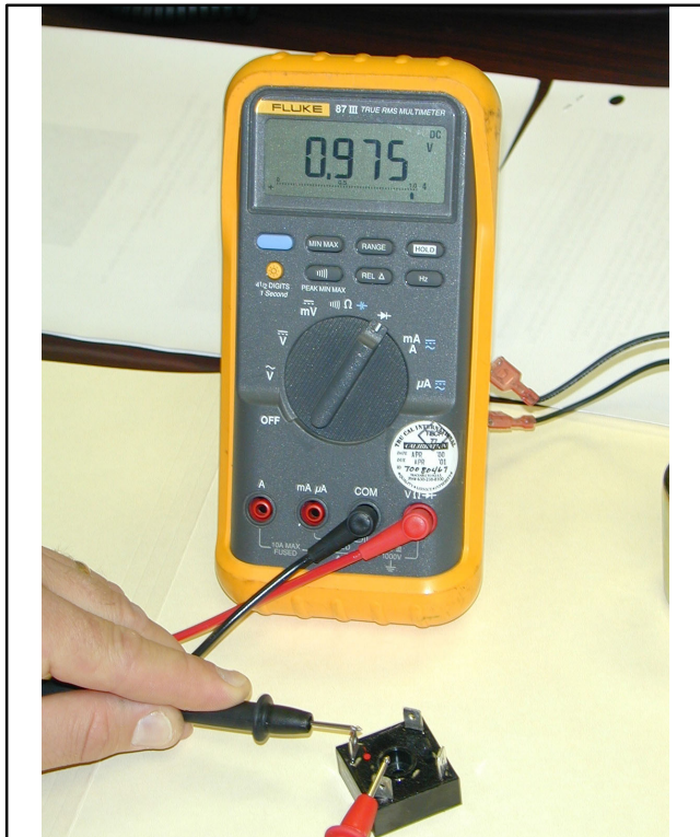
Figure 5-18 Checking Rectifier Diode Operation
