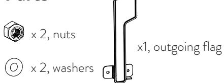
**To attach the flag**, slide it over the threaded rods on the right side of the mailbox, ensuring proper orientation.
