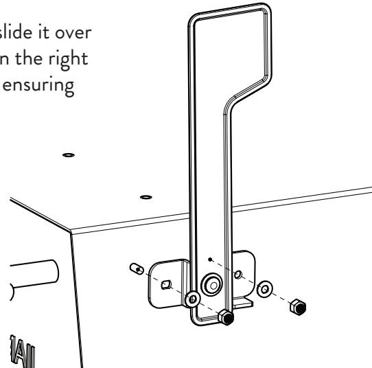
**Then**, place the washers over the rods and secure the flag with the nuts. Tighten the nuts with a wrench.
