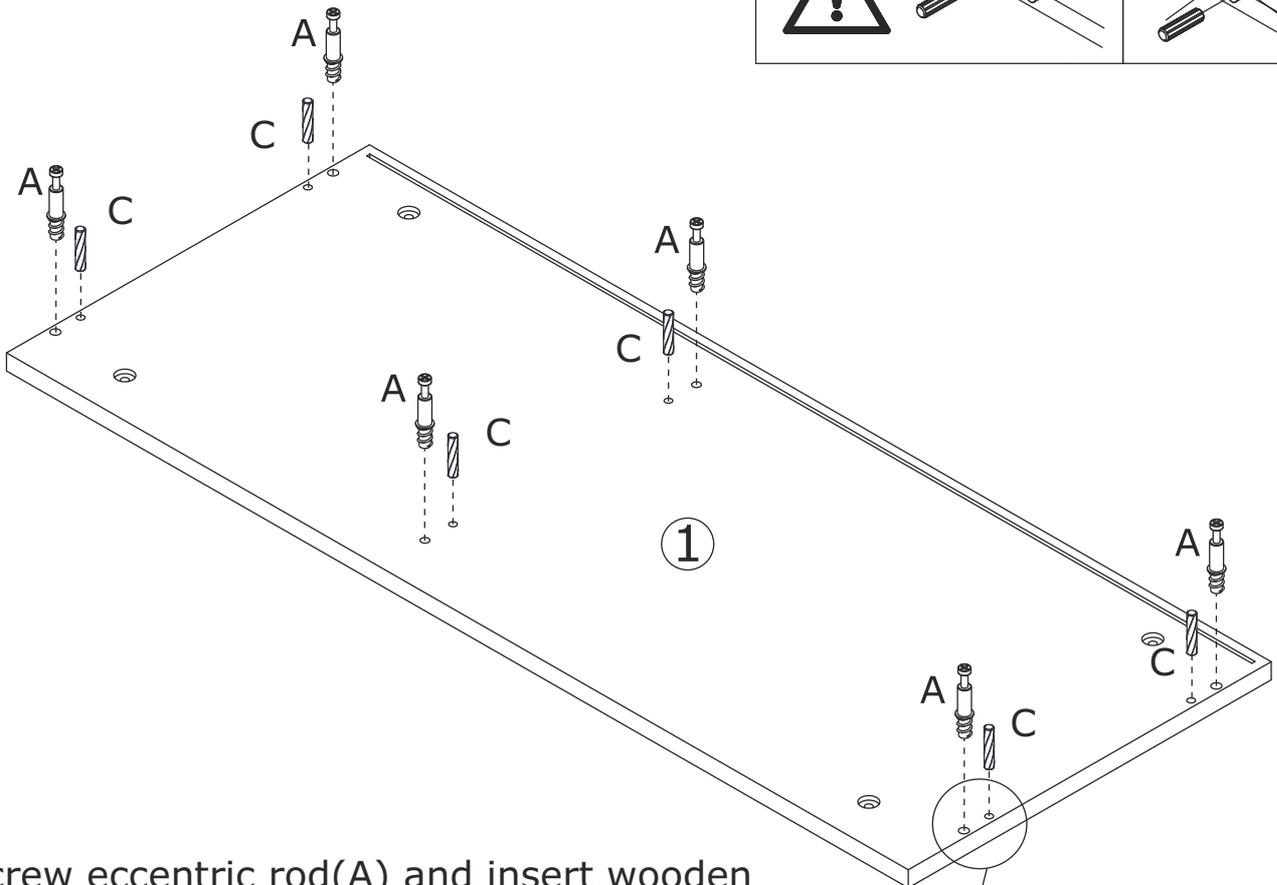
Screw eccentric rod(A) and insert wooden dowel(C) into board 1 as shown.
