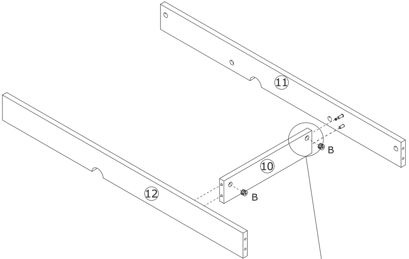
Connect board 10 to board 11 and 12, add cam lock(B) into board 10 and turn clockwise to tighten as shown.
