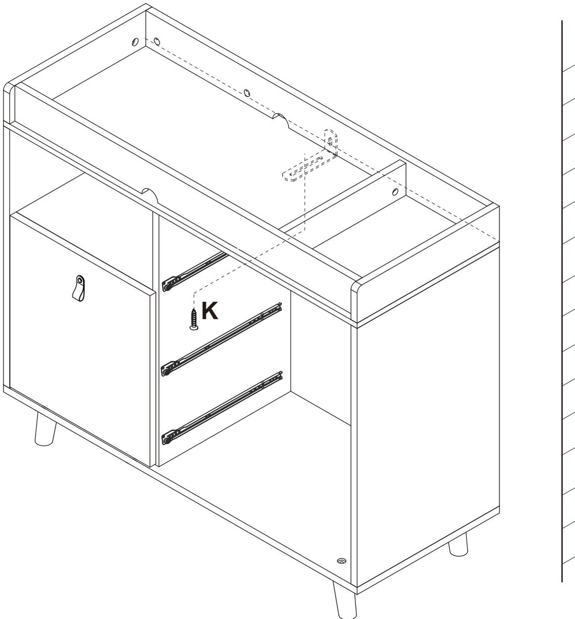
Install anti-tipping device as shown.
