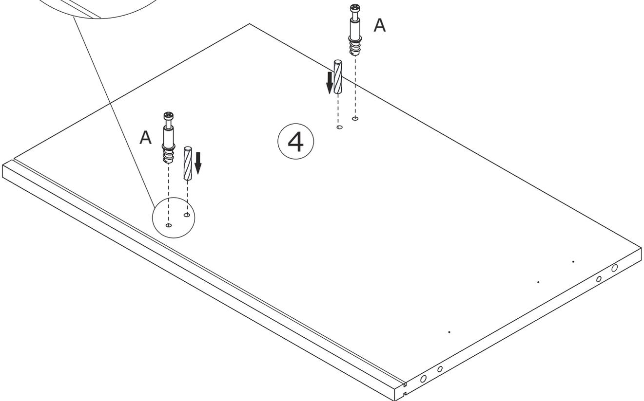
Screw eccentric rod(A) and insert wooden dowel(C) into board 4 as shown.
