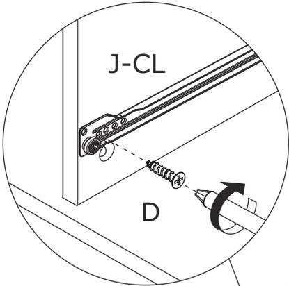
Fix slide rail(J-CL) and (J-CR) to board 4 and 5 respectively with screw(D) as shown.
