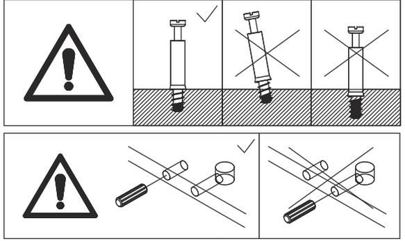
Screw eccentric rod(A) and insert wooden dowel(C) into board 2 as shown.
