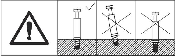
Screw eccentric rod(A) into board 16 as shown.
