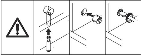
Attach board 22 and 24 to board 21, add cam lock(B) into and turn clockwise to tighten as shown.
