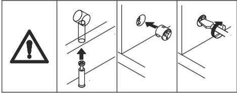
Connect board 3 to board 2, add cam lock(B) into board 3 and turn clockwise to tighten as shown.
