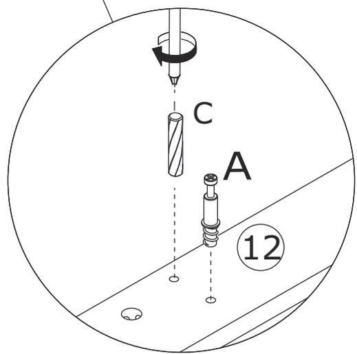
Screw eccentric rod(A) and insert wooden dowel(C) into board 11 and 12 as shown.
