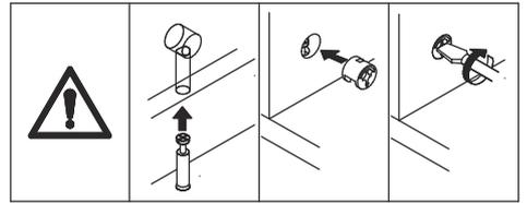
Attach board 5 to board 1, add cam lock(B) into board 5 and turn clockwise to tighten as shown.
