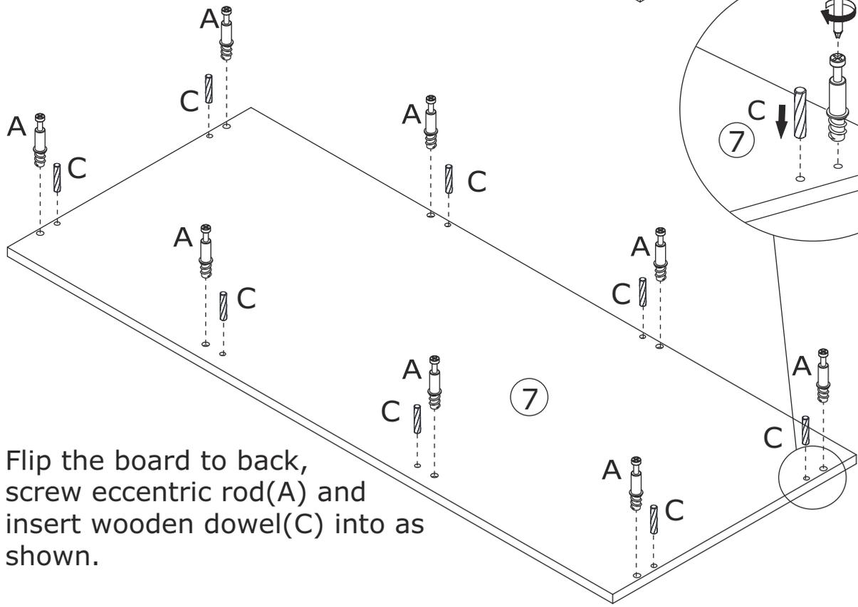
Flip the board to back, screw eccentric rod(A) and insert wooden dowel(C) into as shown.
