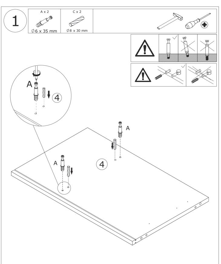
Screw eccentric rod(A) and insert wooden dowel(C) into board 4 as shown.
