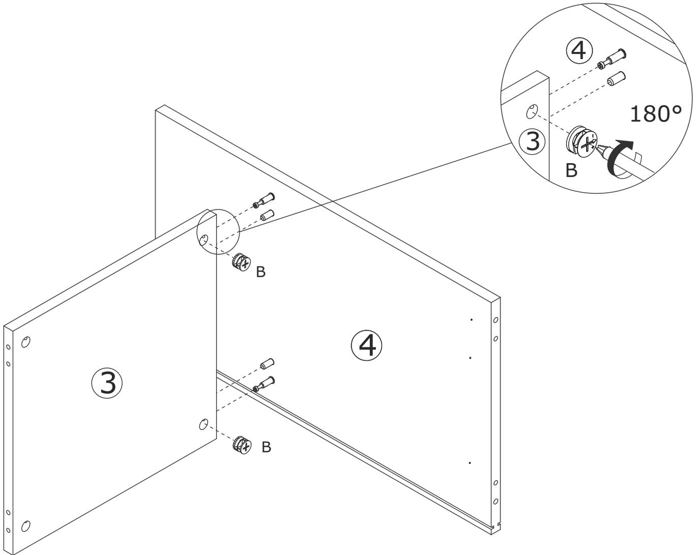
Connect board 3 to board 4, add cam lock(B) into board 3 and turn clockwise to tighten as shown.
