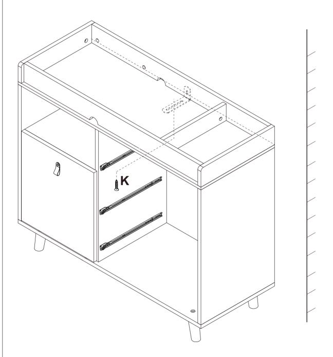
Install anti-tipping device as shown.
