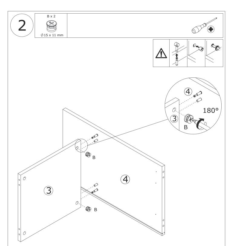
Connect board 3 to board 4, add cam lock(B) into board 3 and turn clockwise to tighten as shown.
