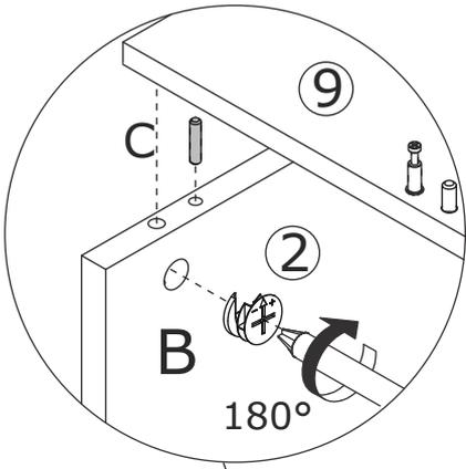
Attach board 7 to the top using wooden dowel (C), add cam lock (B) into board 2, 4, 5 and turn clockwise to tighten as shown.
