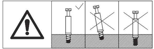
Screw eccentric rod(A) into board 15 and 17 as shown.
