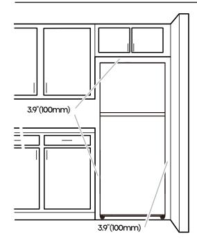
To ensure proper ventilation for your refrigerator, allow for a 3.9"(100mm) space on each side and at the top.
