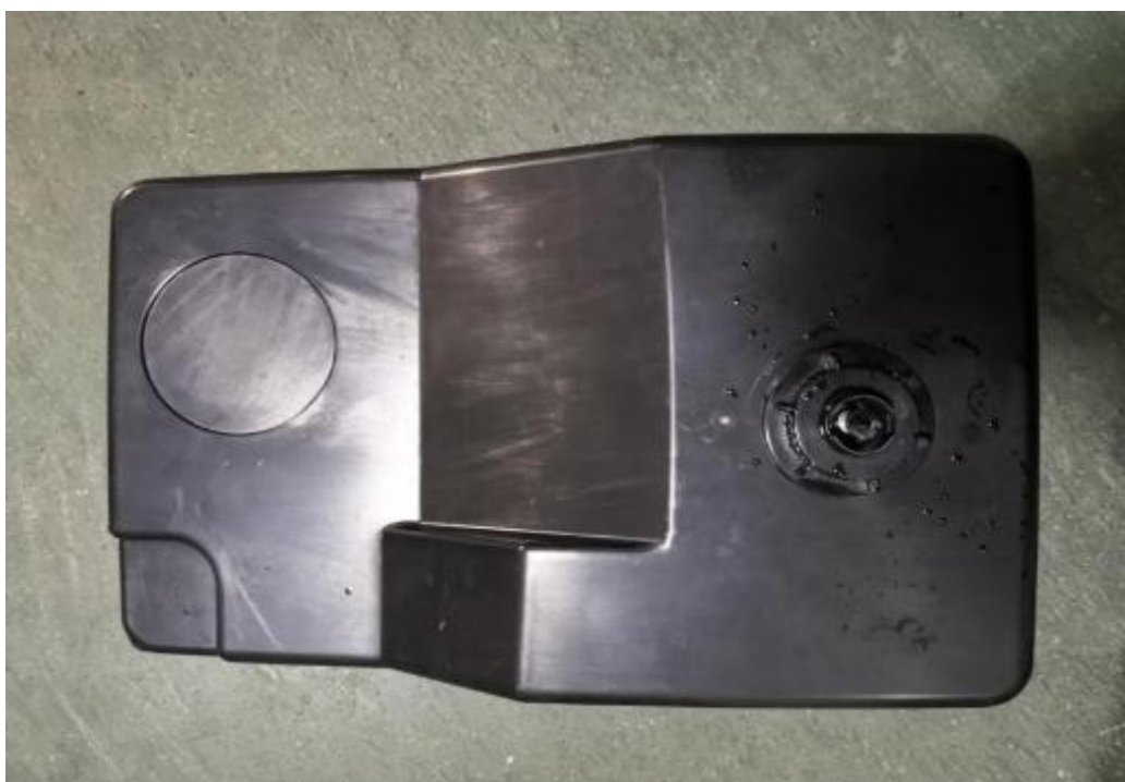
Photo 4.5 - Main water supply tank for HZB-20N, etc (bottom view)
