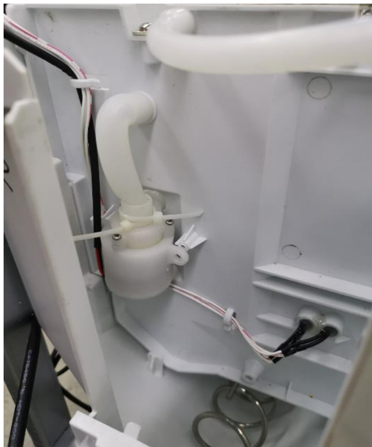
Photo 3.11 - Internal view (Water pump) - HZB-30D
