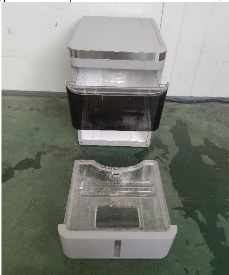
Photo 4.3ap2 - View of door open and remove the water tank for HZB-20FN
