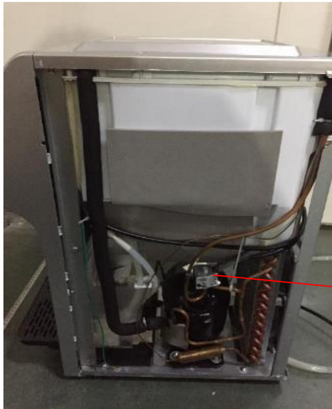
Photo 3.7 - Internal view (right side) - HZB-30D
