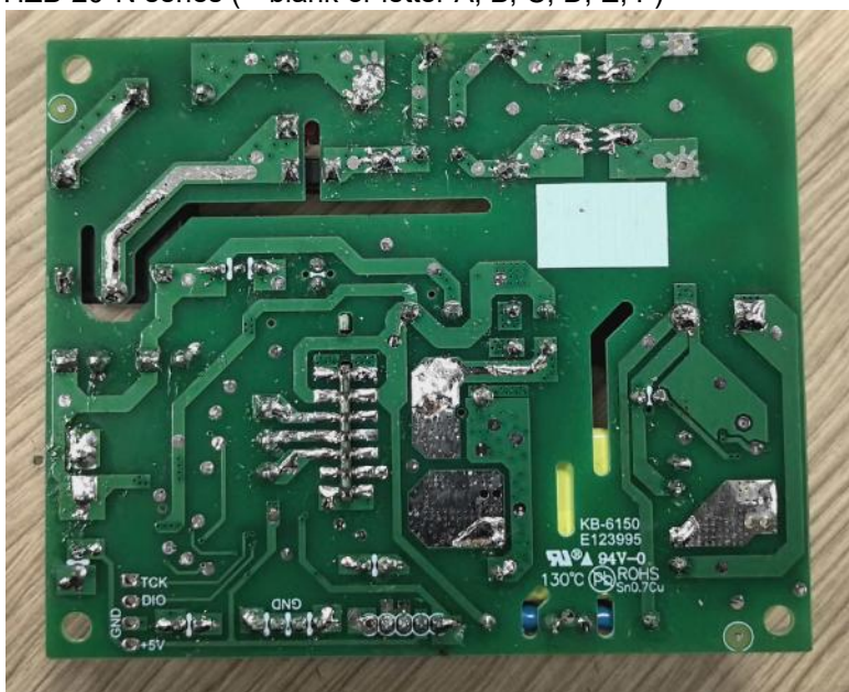
Photo 4.17j - Alternative Main control PCB for HZB-15N* series (*=blank or letter A,B,F,H,G) except for HZB-15DN and HZB-20*N series (*=blank or letter A, B, C, D, E, F)
