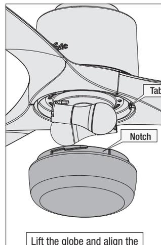
Attach the globe by lifting and turning clockwise one third of a full turn of the glass until it stops.
