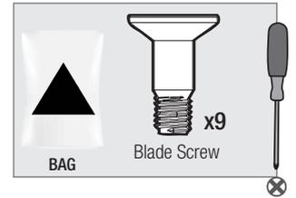
Attach each blade to the blade iron using three blade assembly screws, found in the ▲ hardware bag.
