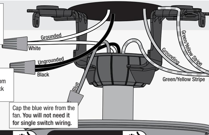
Connect the three grounding wires (green, green/yellow stripe, or bare copper) coming from the ceiling, downrod, and hanging bracket.
