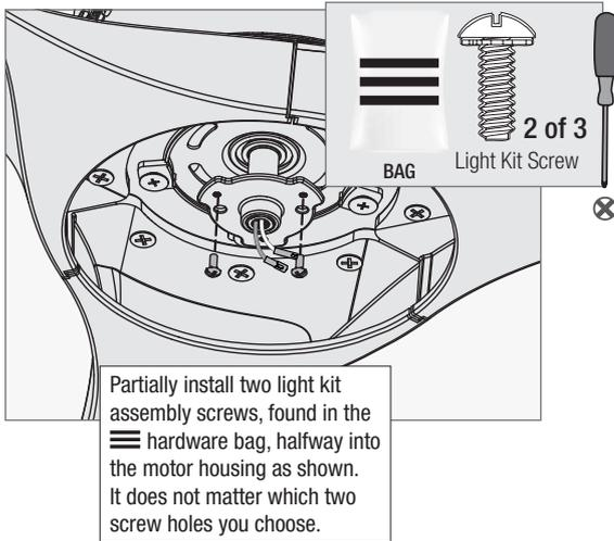
Partially install two light kit assembly screws, found in the hardware bag, halfway into the motor housing as shown. It does not matter which two screw holes you choose.
