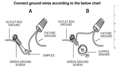
Connect wires according to the below chart
