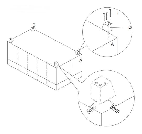
Place the Ottoman (A) on its back on a flat smooth surface. Attach Ottoman Feet (B) to Ottoman (A) with Screw (1) to each corner using a Screwdriver.
