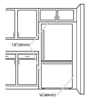
To ensure proper ventilation for your refrigerator, allow for a 1.0" (25mm) space on each side and at the top.
