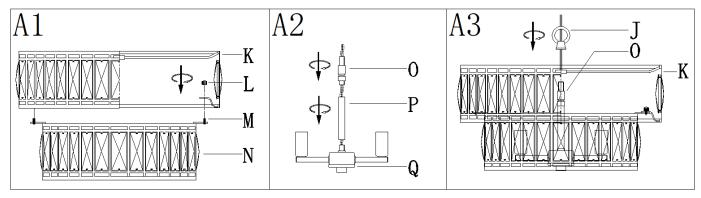
Step A1: Align screws (M) on smaller crystal shade (N) with the holes in bigger crystal shade (K) and then tighten with knob nuts (L).
