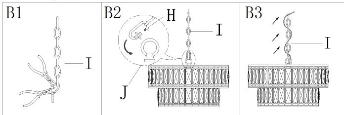
Step B1: By measuring, determine the correct number of links needed for proper hanging height. Using the chain pliers, disconnect and discard the unwanted part.
