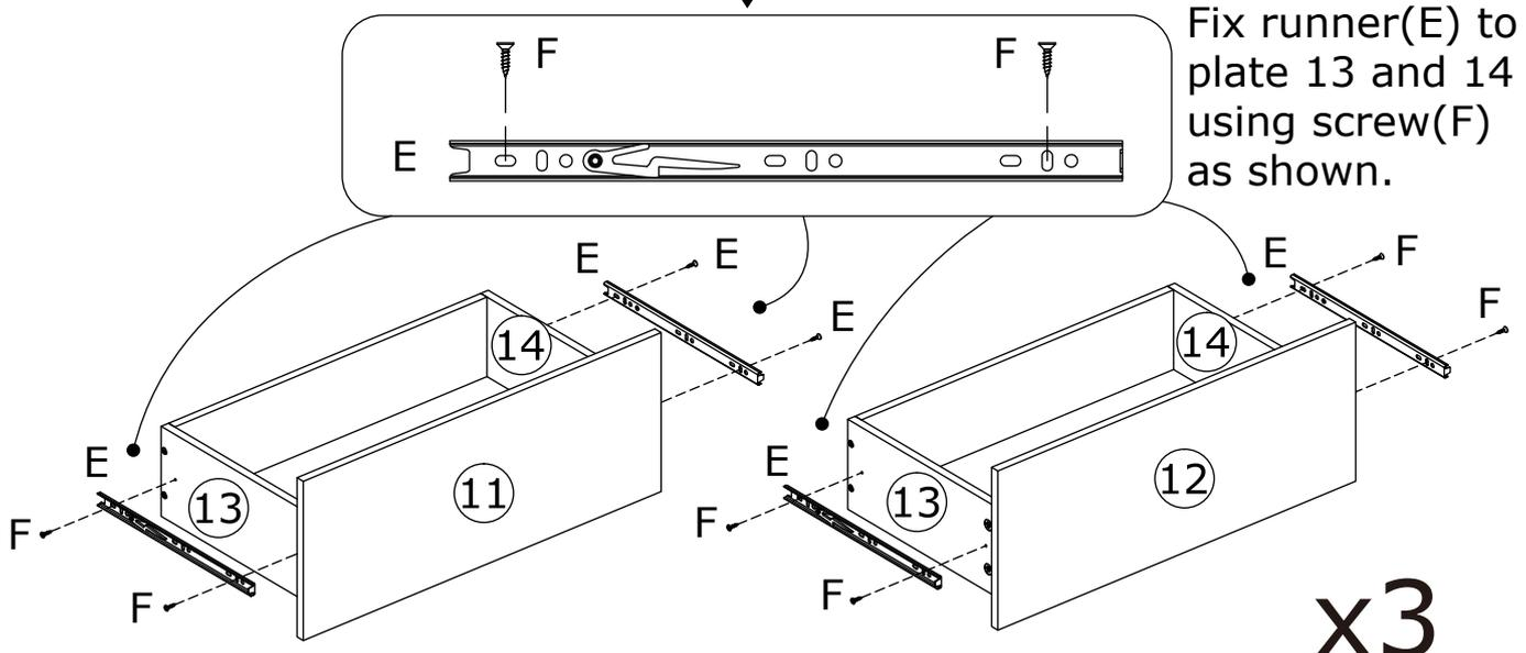
Fix runner(E) to plate 13 and 14 using screw(F) as shown.
