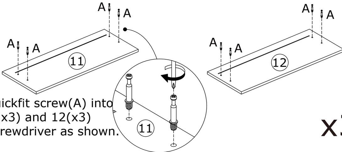
Insert quickfit screw(A) into plate 11(x3) and 12(x3) with a screwdriver as shown.
