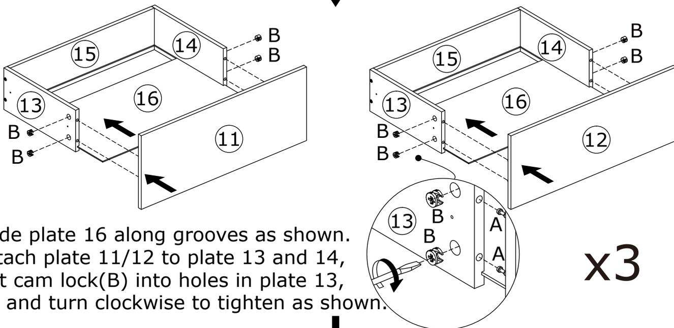
Slide plate 16 along grooves as shown. Attach plate 11/12 to plate 13 and 14, put cam lock(B) into holes in plate 13, 14 and turn clockwise to tighten as shown.
