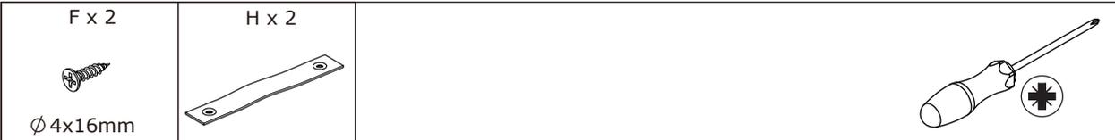
Fix cloth trip(H) to back of the item using screw(F) as shown.
