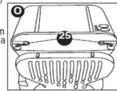
Remove the two screws (25) shown in (figure O) and lift off the battery housing.
