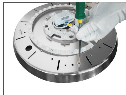
Step 4. Remove the main engine chassis screws.
