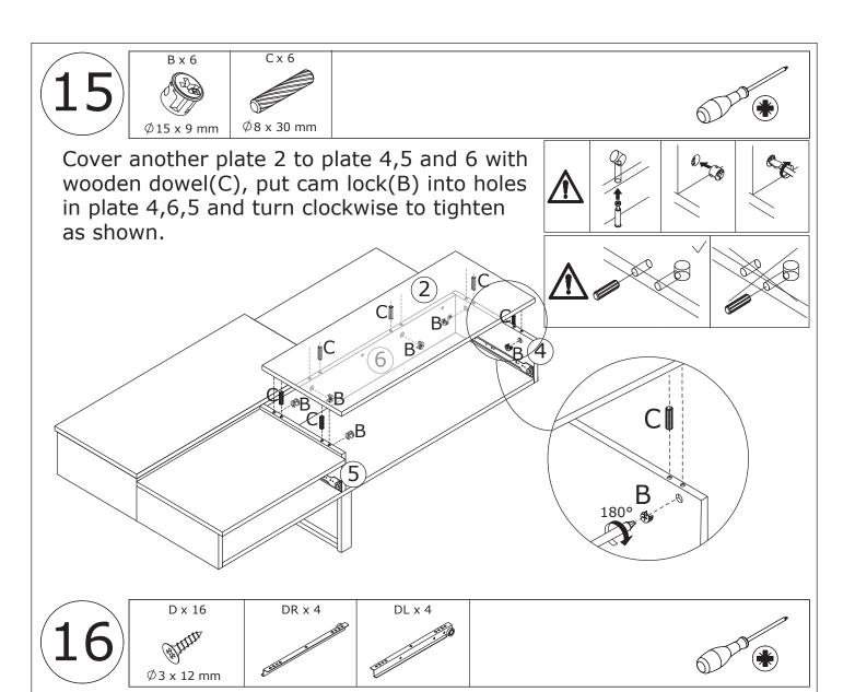
Fix runner(DL) and (DR) to plate 12 and 13 respectively using screw(D) as shown.
