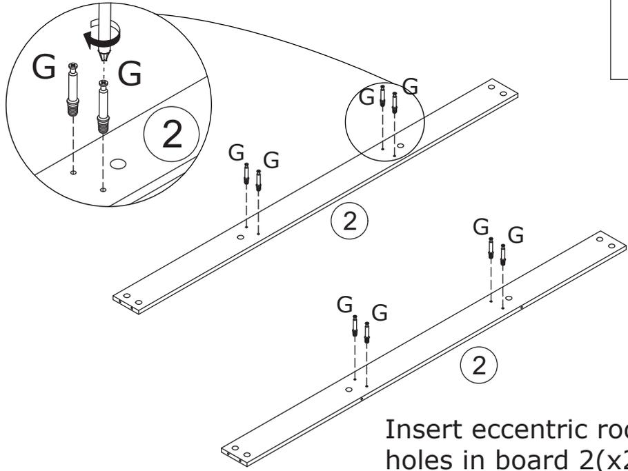
Insert eccentric rod(G) into corresponding holes in board 2(x2) as shown.
