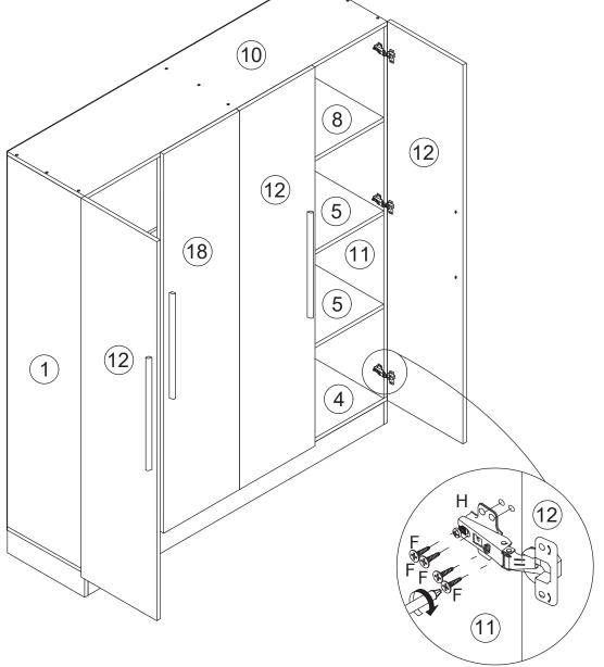
Attach another two board 12 to board 1 and 11 by fixing hinge(H) with screw(F) as shown.
