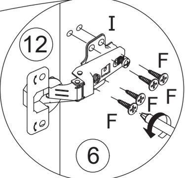
Attach board 12 to right of board 6 by fixing hinge(I) with screw(F) as shown.
