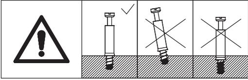
Insert eccentric rod(G) into corresponding holes in board 4 as shown.
