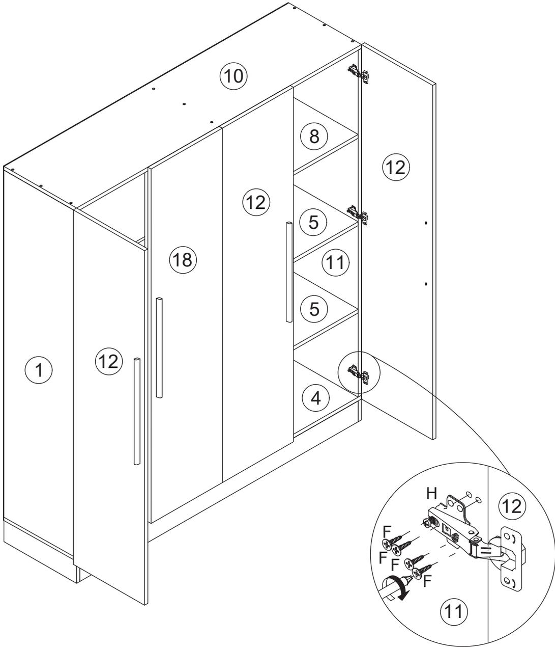
Attach another two board 12 to board 1 and 11 by fixing hinge(H) with screw(F) as shown.
