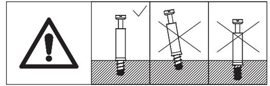
Insert eccentric rod(G) into board 16(x2) as shown.
