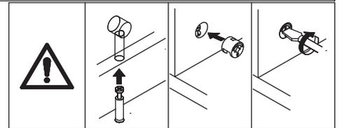
Attach board 16 to board 2, put cam locks(E) into holes in plate 2 and turn clockwise to tighten as shown.
