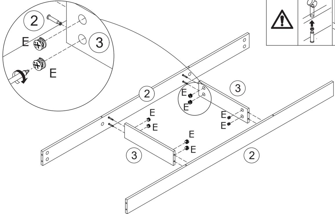
Connect plate 2 with plate 3, put cam locks(E) into holes in plate 3 and turn clockwise to tighten as shown.
