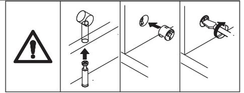
Attach the frame to plate 4, put cam locks(E) into holes in plate 2,16 and turn clockwise to tighten as shown.
