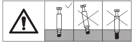
Insert eccentric rod(G) into corresponding holes in board 6 at first. Flip the plate, insert quickfit screw(G) as shown.
