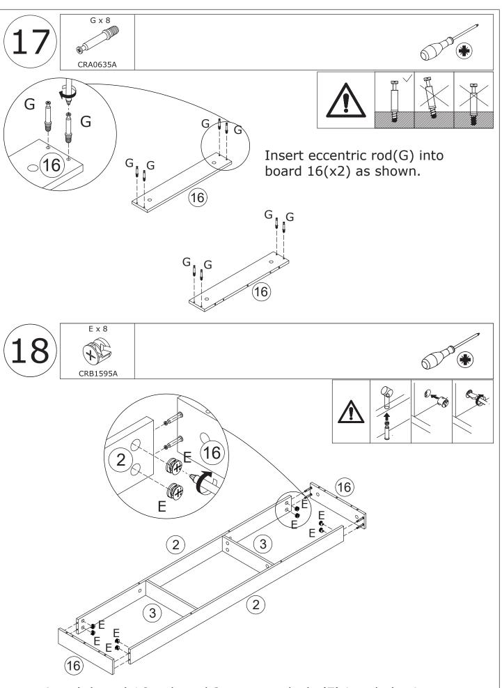
Attach board 16 to board 2, put cam locks(E) into holes in plate 2 and turn clockwise to tighten as shown.
