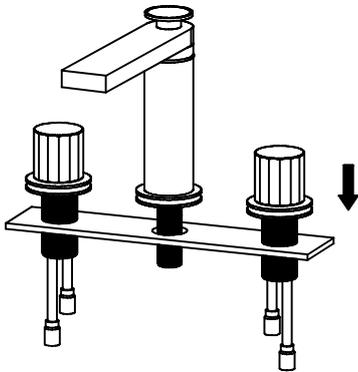
2. Re-install the rubber washer followed by the metal washer and lock-nut. Hand tighten then tighten further using a screw driver to tighten lock-nut screws
