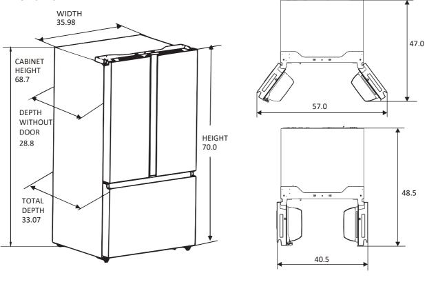
Keep enough clearances between the appliance and its surroundings to ensure the function of the appliance.
