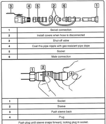
To disconnect, push sleeve back and pull out plug. (This automatically shuts off gas.)
