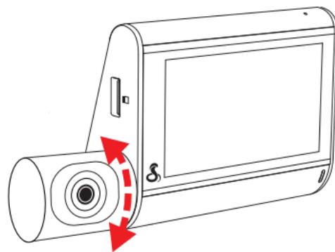
Rotate the interior cam so that it captures a view of the driver and passengers.
