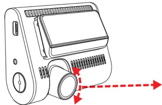
Rotate front camera lens so that it is parallel with the road.
