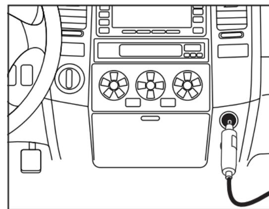
Connect the USB-C cable into the dash cam and plug the power adapter into the vehicle's 12V port
