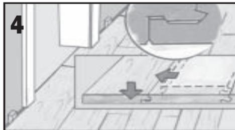
Slide panel into place horizontally and slot in profile. Use these modified planks under doorframes, radiators, cabinet fronts, etc. Use the pull bar to slide the planks where needed.
