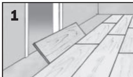
Some long edge joints cannot be installed using a 12° angle.
