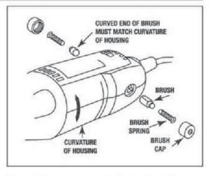
by rotating cap counter-clockwise and check each brush.
