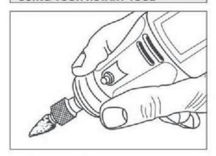
The first step in learning to use the Rotary Tool is to get the "feel" of it. Hold it in your hand and feel its weight and balance. Feel the taper of the housing. This taper permits the Rotary Tool to be grasped much like a pen or pencil. The #470 Variable Speed tool has a unique comfort grip on the nose and back seating, which allows the user added comfort and control during use. You can feel the difference!
