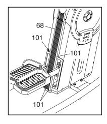
Next, turn the Large Pulley (21) until a Pulley Magnet (104) is aligned with the Reed Switch (116). Then, slightly loosen the M4 x 22mm Screw (107), slide the Reed Switch slightly closer to or away from the Pulley Magnet, and then retighten the Screw.
