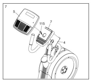
Avoid pinching the wire. Attach the Console (5) and the Console Cover (7) to the Console Bracket (4) with four M4 x 22mm Screws (107). Start the two upper Screws first, and then start the two lower Screws; then, tighten all four Screws.
