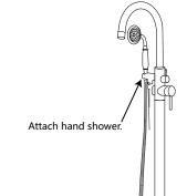
9. Once installation is complete, turn on the main water supply. Turn the faucet on and allow the water to flow for 60 seconds. Check for any leaks, and that hot and cold water are running appropriately. Divert the water to the hand shower and allow the water to flow through the hose for approximately 60 seconds
