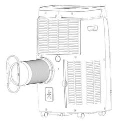
**Step 6:** Adjusting the length of the flexible exhaust hose, to make sure the distance between the unit and the window will be more than 70cm, and the height from exhaust hose to the floor will be more than 90cm. And avoid bends in the hose. Then place AC near an electrical outlet.
