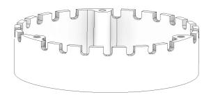
After assembling all the burner pieces, place it into the bottom of the firepit. Align the burner studs with the holes in the bottom of the firepit. NOTE: If a replacement Burner Kit (893653) is needed please call customer service.
