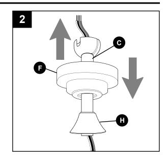
3. Slip downrod (C) into motor housing yoke, align holes and re-install pin (D) and clip (E). Tighten set screws in motor housing yoke and then tighten preassembled nut on one of the set screws. Then, slide yoke cover (H) and canopy (F) down until they rest on top of motor housing assembly (I).
