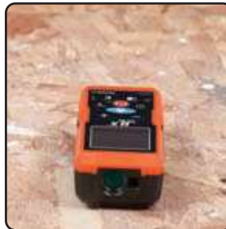
Cal3: Rotate 180°, LCD towards you.
