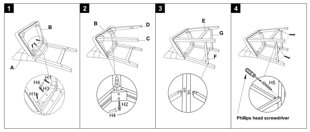
Step 1: Assemble seat cushion (B) with chair back (A).Using Wrench (H4) to lock with 5\*bolts (1\*H3 & 4\*H1).
