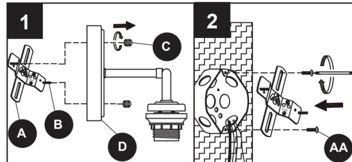
Attach A to outlet box using AA. Temporarily place D through B determine amount of adjustment necessary B.
