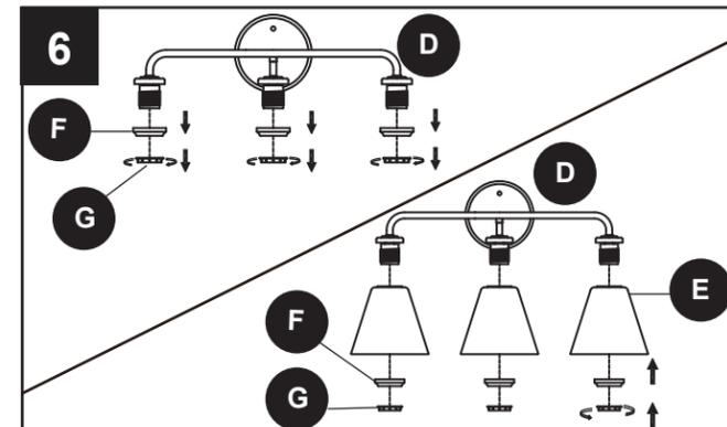
Unscrew sockets rings G, remove the metal rings F from sockets on fixture body D. Attach glass shades E over the sockets. Place the metal rings F.
