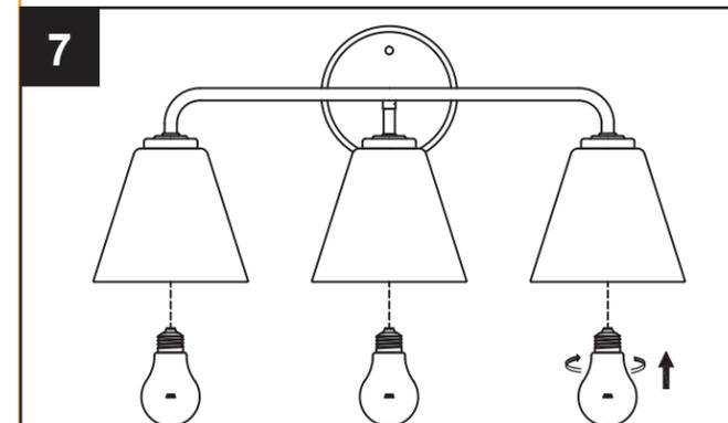
Install light bulbs (not included). Use 60-watt max. standard-base incandescent bulbs or CFL/LED equivalents.
