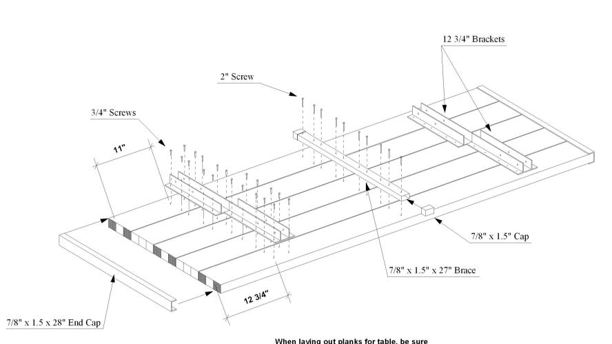
When laying out planks for table, be sure to use 5 planks from Box 1. The planks in Box 1 have holes that are not evenly spaced from each end. Lay out the planks as seen above.
