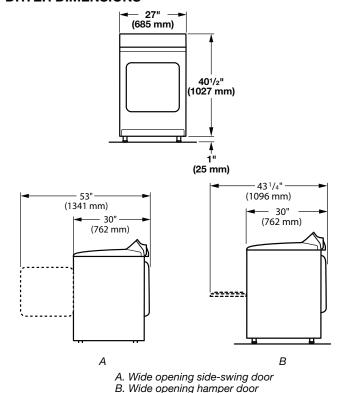
\*Most installations require a minimum 6" (152 mm) clearance behind the dryer for the exhaust vent with elbow. See "Venting Requirements."
