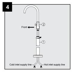
Screw the standpipe (1) onto the mixer (2) by hand. Turn in a clockwise direction until it is tight. Note: Do not to reverse the cold and hot supply lines.
