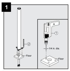
Drill a hole min 2 1/4 in. diameter-max 2 9/16 in. diameter in the floor with an electric drill (1). Mark the locations for the screws with a pencil (2). Then drill three holes 1/4 in. diameter for the screws in the floor with an electric drill (1).
