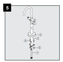
Place the assembly with the flexible supply lines (1) through the prepared hole and then holding the escutcheon (2), secure the standpipe (3). Note: If mounting into wooden floor, secure the standpipe (3) using screws (4) only (wall plugs are not needed). If mounting into solid floor, mark the position of holes first and then secure the standpipe (3) using anchors (5) and screws (4). Where requried ensure correct anchors for your floor type are used.
